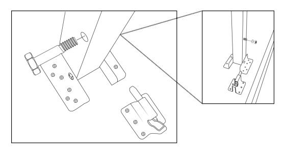
When attaching the legs together, place the gray plastic piece between the two metal frames:
