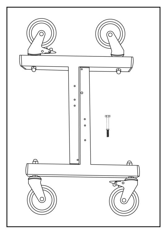
One leg has an extra hole for the lock bolt
