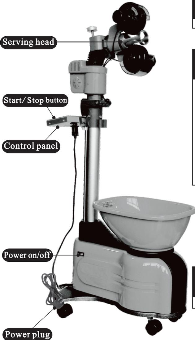
**1** Insert the plug into the power supply. Switch on the robot and the power indication light will turn on.
