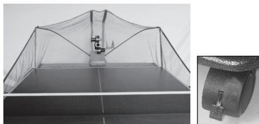
3. Move the robot close to the table and lock the casters. Fasten the velcro of the ball collection net to the middle net of the table.
