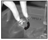
ATTACH BALL COLLECTOR PLATE Using the three Phillips Head screws provided, attach the Ball Collector Plate to the bottom of the robot body as shown. The robot body has a round and a rectangular locating pin that match up with similar shaped holes in the plate.
