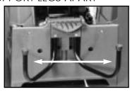
JOIN NET SUPPORT TUBES Turn the robot around 180° so the Net Support Tubes are now facing you. Grasp the second tube from the right and pull up, removing it from its storage hole. Place the bottom of this tube into the top of the first tube on the right as shown. Repeat on the left side.
