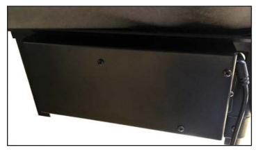
Now hook the Tablet Holder onto your Control Panel Bracket. If you haven't done so already, we recommend the use of a long Velcro strip (that came with your robot) to secure the Control Panel Bracket onto your table. This will help prevent knocking the tablet off the table, which could then crack its screen or otherwise damage it.
