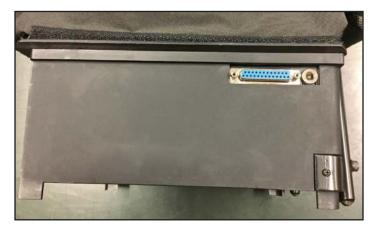
Take the Power Control Board and match its serial port with the serial port on the Base. Press down on the metal cover above the serial port until you feel the two halves of the serial port are fully mated together. Also be sure to not cover the power port with any part of the metal cover (see photo below).
