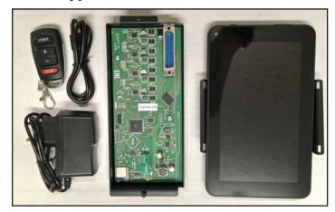
The above photo shows the components included in the kit. You will receive an Android tablet preloaded with the Amicus app and with the Tablet Holder preattached, a Power Control Board attached to a metal cover, screws to attach the cover, a Tablet Power Supply, a Remote Switch Key Fob, and a USB Micro charging cable (alternative method for charging the tablet). You will also receive the Prime Owner's Manual (not pictured).
