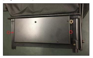
Next, using a power screwdriver, screw the two #1 Phillips screws (indicated by red circles above) into the side of the Base. These screws are self-drilling, so it is not necessary to drill a pilot hole. As the screw approaches full insertion, be careful not to screw too forcefully, which can strip out the threads in the plastic.
