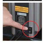
The robot is powered by standard US home current (120V). Make sure the power cord is securely plugged in. On/Off switch is located on the backside of the robot. Turn off and unplug the robot when not in use.
